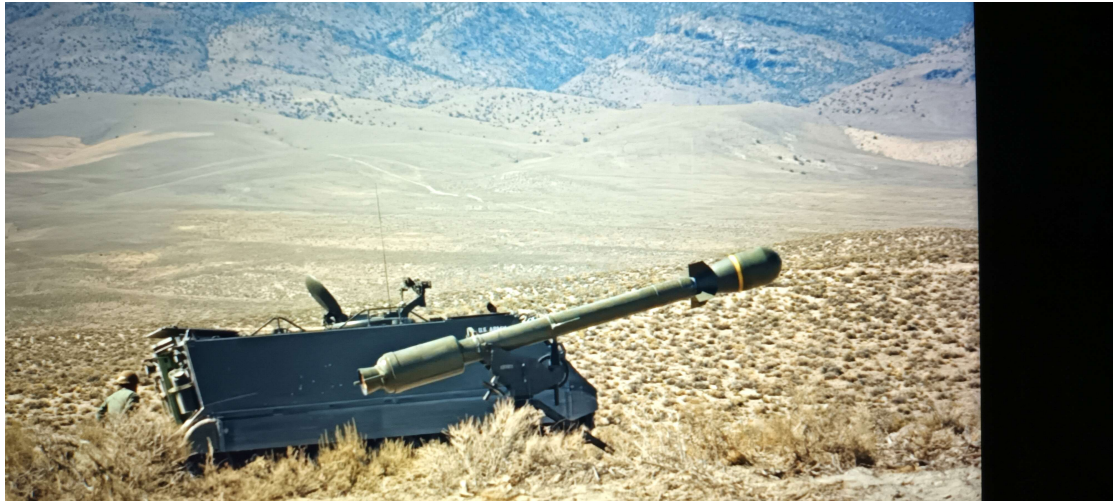
ABOVE: 22 ton of TNT nuclear yield Little Feller II on stand beside an APC (used as shelter).
